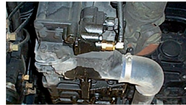
All leaks from the engine, gearbox and differential, hydraulic suspension and dampers
