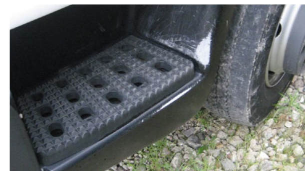
Scratches that can be felt with your nail or surface > 45 \text{ cm}^2 (equivalent to a credit card)
