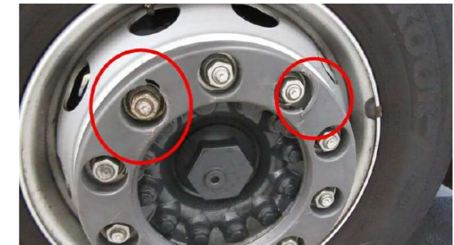
Wheel covers: Deformed, broken, material missing or removed
