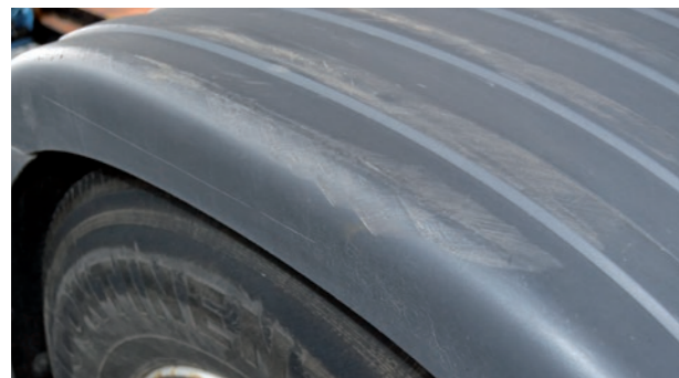
Slight surface scratching
