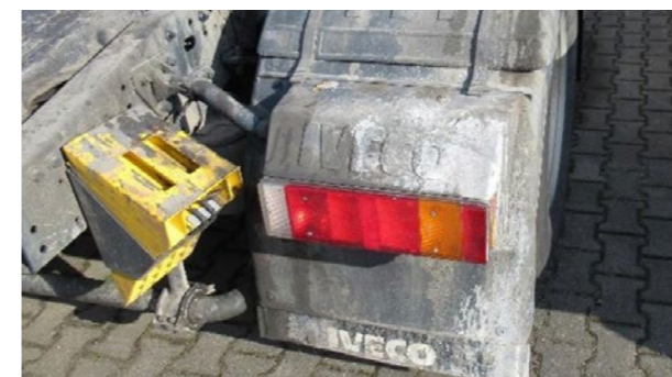
Deep discolouring due to chemical elements
