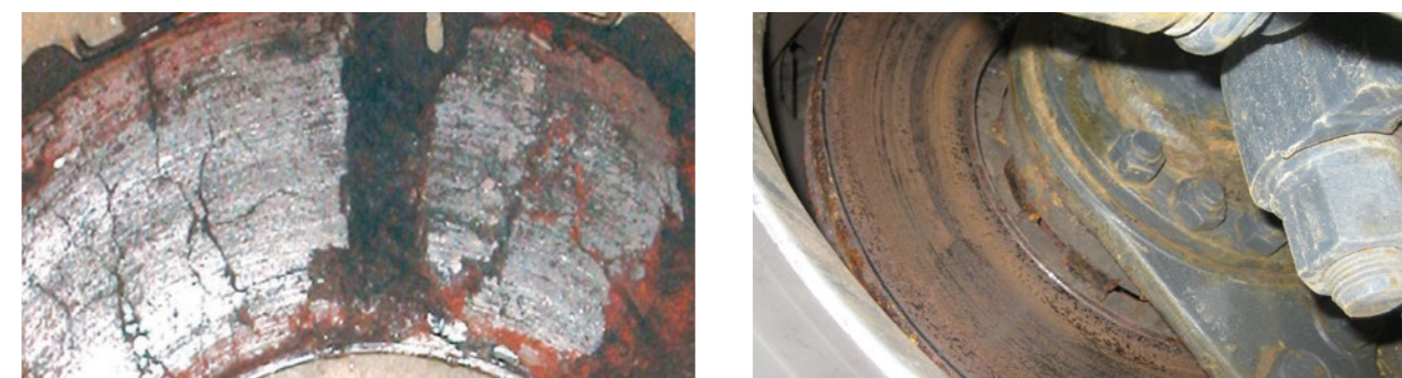
Rusted, ground, worn brake discs
