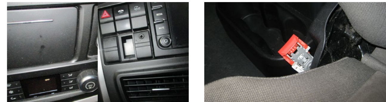
Control parts, seat or trim parts missing, broken or pierced
