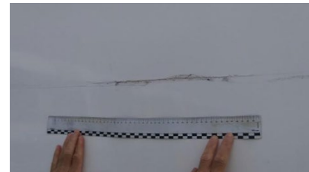
Side panels: Scratch with removal of material \geq 20 cm within economic repair. Option to paint half panel
