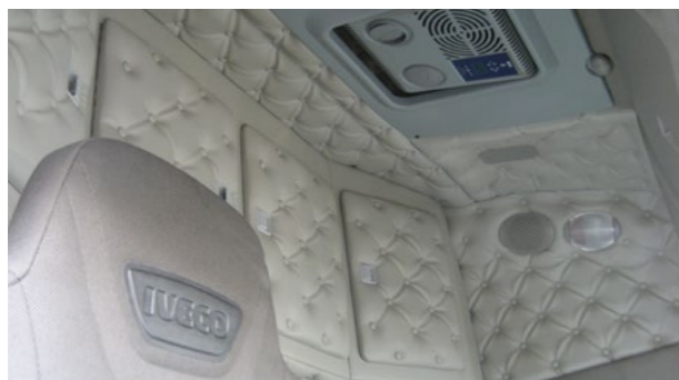
📋 Slight decolouration due to sun rays
