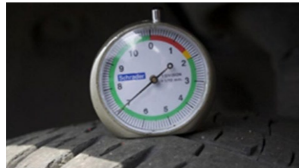
Tyres: Base of groove depth \geq 7 mm (CONFORMS) Note: The wear of the tyres is measured in the most worn groove on the tyre.
