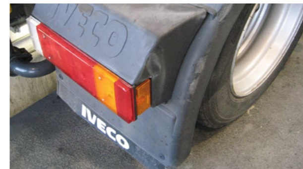
Deep scratches and deformation
