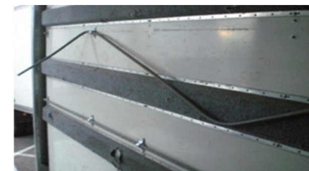
↻ Upholstery and rods: Rods, fastenings, upholstery missing or deformed beyond economic repair
