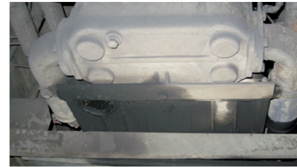
Leaks from the steering gear and power steering pump
